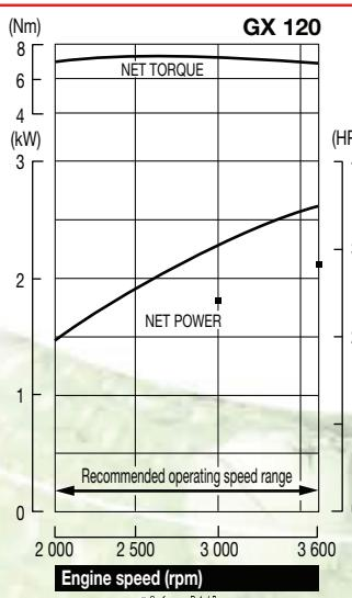
The power rating of the engine indicated in this document is the net power tested on a production engine for the engine model and measured in accordance with SAE J1349 at a specified rpm. Mass production engines may vary from this value. Actual power output for the engine installed in the final machine will vary depending on numerous factors, including the operating speed of the engine in application, environmental conditions, maintenance, and other variables.
