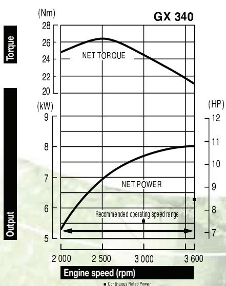
The power rating of the engine indicated in this document is the net power tested on a production engine for the engine model and measured in accordance with SAE J1349 at a specified rpm. Mass production engines may vary from this value. Actual power output for the engine installed in the final machine will vary depending on numerous factors, including the operating speed of the engine in application, environmental conditions, maintenance, and other variables.
